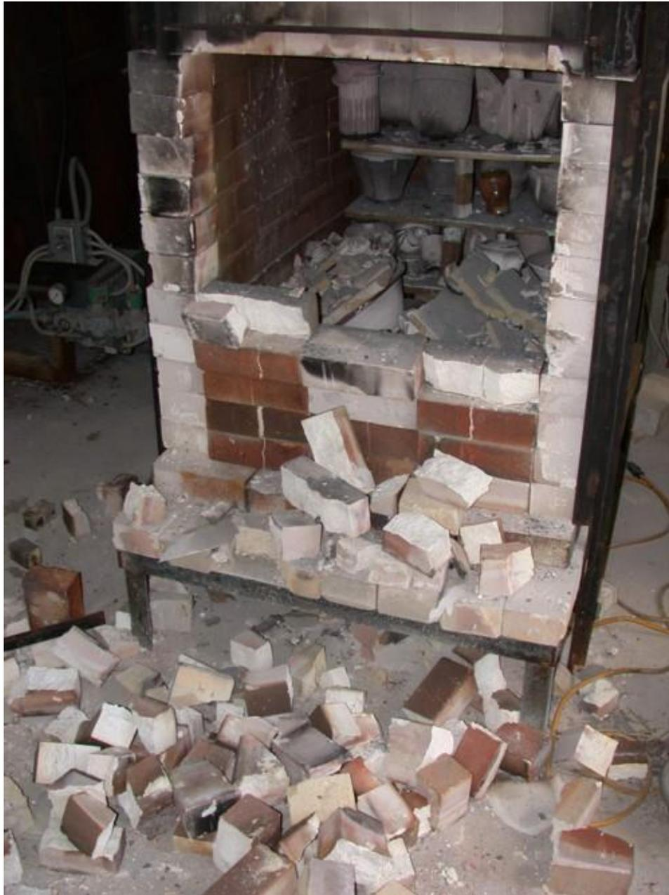
This is Nils Lou's small kiln that exploded because of a damp Advancer shelf. A student mistakenly washed an Advancer kiln shelf in water, and let it soak to clean it. Here are the results. Everything in the kiln must be dry, totally dry.
