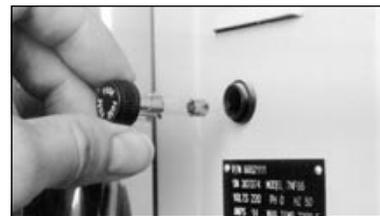
The kiln switch box fuse holder.
