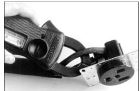
The ammeter attaches to only one hot wire. Be sure breaker is shut off before you remove the receptacle cover.
