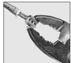
Tighten loose push-on connectors by squeezing gently with pliers.
