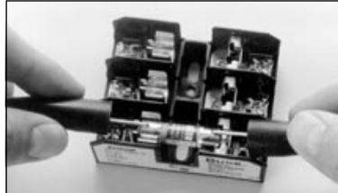
Test a high amperage fuse with an ohmmeter. You can test the fuse without removing it from the fuse holder.
