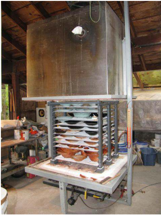
My Doorless Fiberkiln with Advancer posts and shelves. $28 to fire with 4 hour soak.
