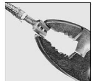
Tighten loose push-on connectors by squeezing gently with pliers.
