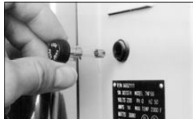
The fuse holder is on the side of most kiln switch boxes.
