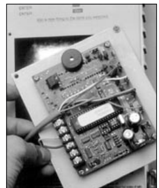
Disconnect power before removing the board from the switch box.
