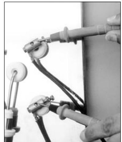
The ohmmeter sends an electric current through the element. If the element is broken, the meter will show an OPEN circuit.
