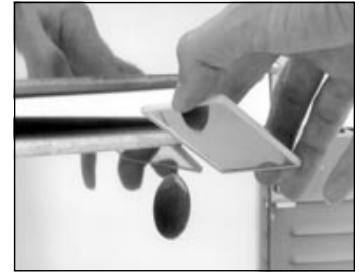
With a mirror, you can detect moisture escaping from the kiln. Keep the lid in the vented position until the mirror no longer fogs.
