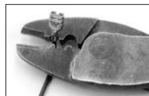
The indent on the crimping tool goes on the side opposite the seam of the connector. Test the crimp by pulling on the wire firmly.
