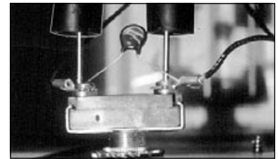
Testing a door switch with an ohmmeter: this switch mounts inside the main switch box.
