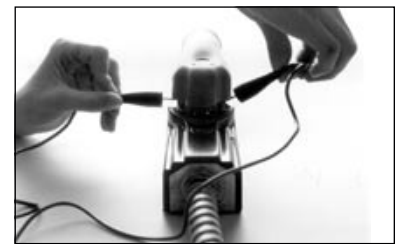
While the kiln is firing, measure voltage at the cord plug. Be sure not to touch the metal part of the voltmeter probes.
