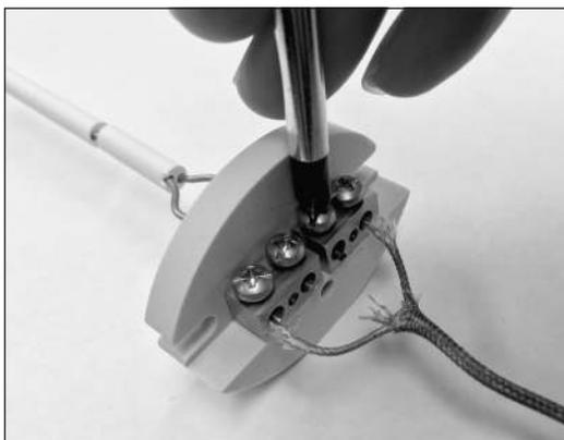
Before fastening the thermocouple connection block to the kiln, tighten all four screws.
