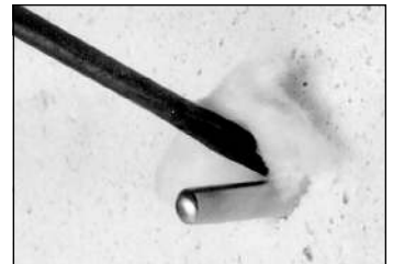
10. If the thermocouple hole is 1/2", stuff ceramic fiber around the thermocouple.
