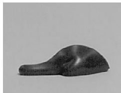
Overfired or "puddled" cone.
