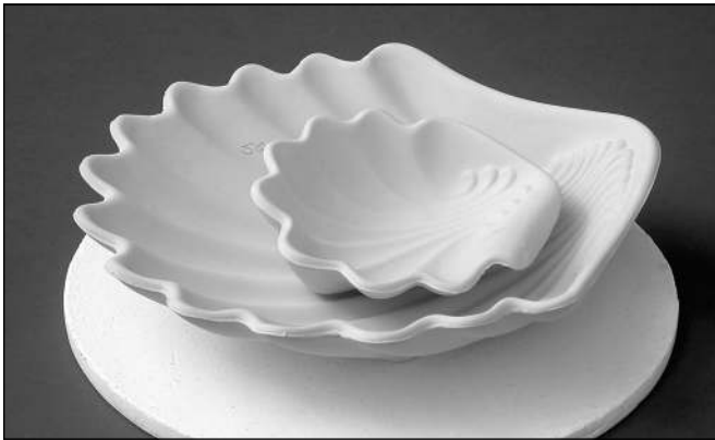
"Nested" greenware must not be loaded too tightly.
