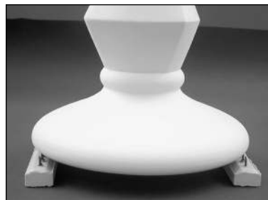
Bar stilts support longer pieces and pieces with a large hollow base.
