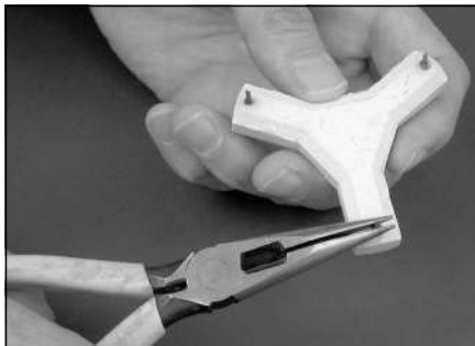
Straightening a stilt point.
