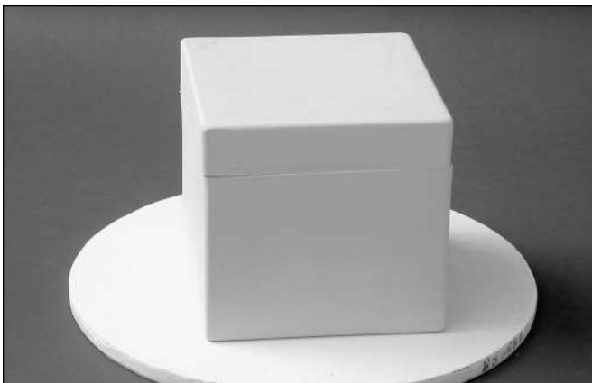
Fire greenware box and lid together to ensure a good fit.
