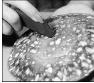
Removing stilt marks with a stilt stone.
