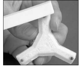
Cleaning stilt wire with a stilt stone.
