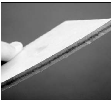
A cross-section of the fired clay shows a black line. This is carbon that did not burn out completely.
