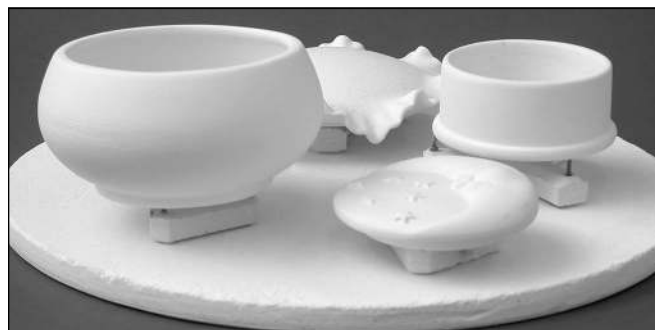
In the greenware firing, a bowl and lid are fired together. In the low-fire glaze firing, they are kept separate as shown above.
