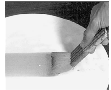
Applying separator to the shelf.
