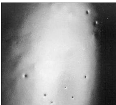
Pinholes from underfired bisque.
