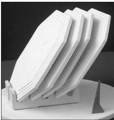
Firing plates vertically minimizes the chance of debris falling on them during firing.
