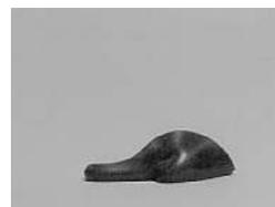
**Note:** Do not be overly concerned with achieving an exact 6 o'clock bend. The difference between a 3 o'clock and a 6 o'clock bend is only a few degrees of temperature.
