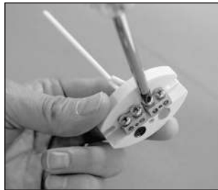
The S-type thermocouple must extend into the firing chamber 1/2" - 3/4".
