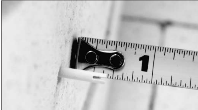
The S-type thermocouple must extend into the firing chamber 1/2" - 3/4".
