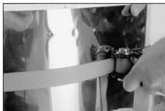
8 Reinstall the LiteLid assembly onto the back of the kiln. Attach the bottom of the spring to the LiteLid. Models without lid spring: Reinstall the screws in the lower hinge.
