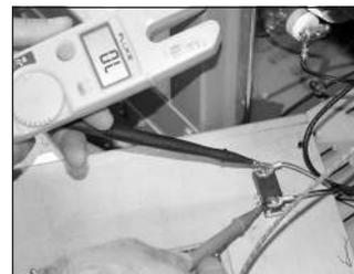
Testing the door push-button safety switch.
