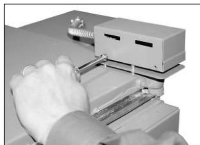
The door rotary safety switch is mounted on top of the door hinge shaft.
