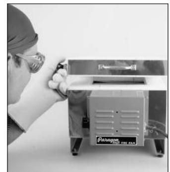
Then close the lid. Wear firing safety glasses and protective gloves. Lift the side handle on the lid.
