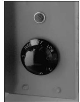
The pilot light above the switch serves as the pointer mark for the numbers on the switch knob. As you turn the knob from LOW through MED and higher, the kiln will fire progressively faster. When you turn the switch to HIGH, the element will stay on continuously. The switch settings do not correspond to a particular heating rate or temperature hold.
