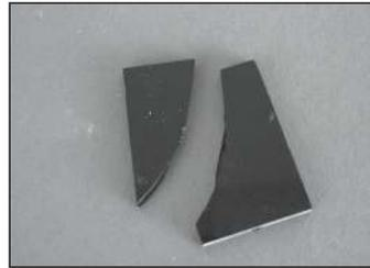
*The glass was removed too soon from the kiln.* Allow the glass to cool at least 45 minutes before lifting the kiln top and removing the piece.
