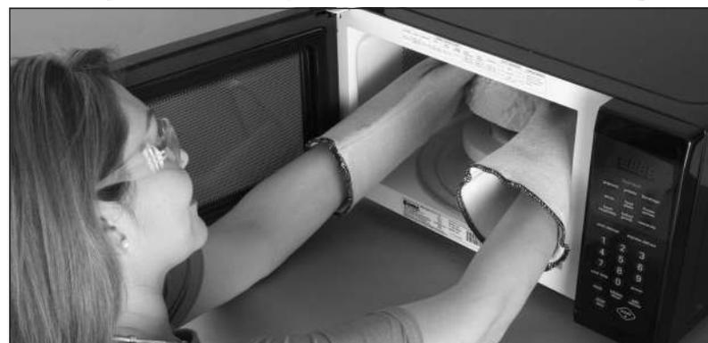
Wear safety glasses and stay at arm's length when checking the glass visually.
