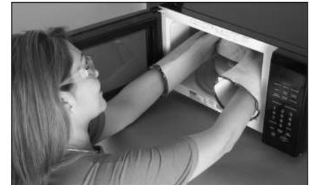
Wear safety glasses when visually checking the glass in the kiln.
