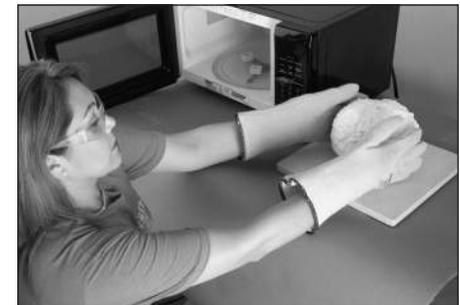
Remove the kiln right after the firing is finished. Wear heat-protective gloves.
