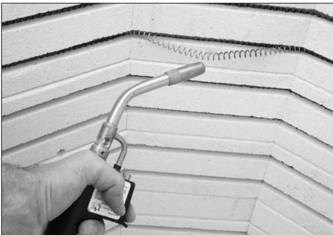
torches. Turning them on and off is awkward. You first turn a knob to start the flow of propane and then hold a match under the nozzle.
