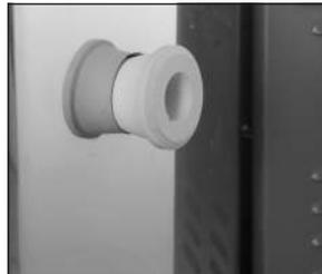
When looking through the peepholes, always wear firing safety glasses, which are available from Delphi. They protect your eyes from the bright glare of the firing chamber and make it easier to see the cones at high temperatures.
