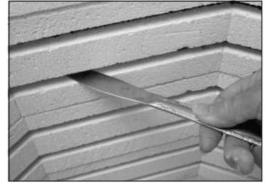
**Note:** Don't force the element into the groove corners. If the element won't fit easily, lengthen it with automotive snap-ring pliers. Stretch the space between the coils just a little where the element fits into the wall brick corners. It should then easily seat into the corners.
