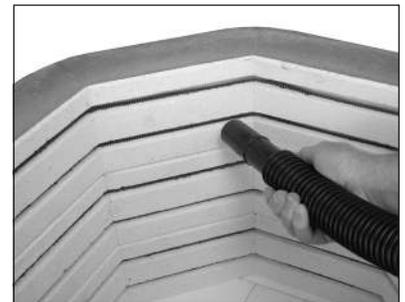
You can use a plastic vacuum nozzle, but do not touch the firebricks with the nozzle.
