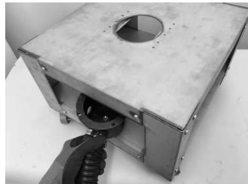
**3** Place the gasket that came with the vent over the vent cup as shown at right.
