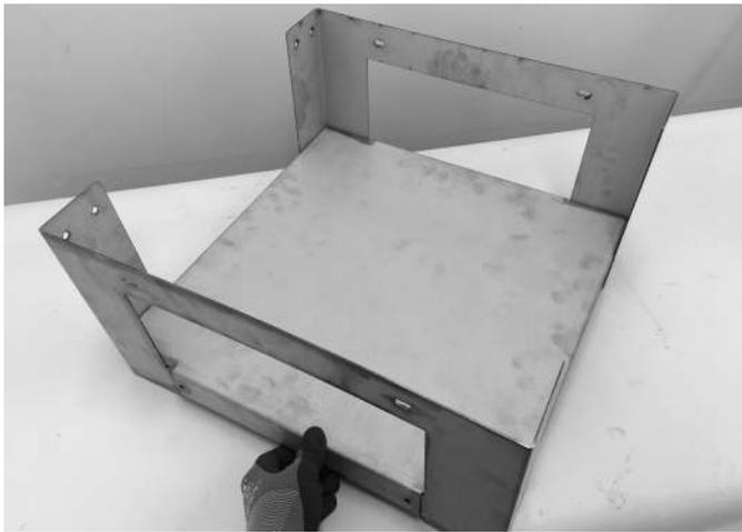
**3** Lay the top shelf (the one with the hole in the center) over the side frames. The short tabs slide over the outside of the side frames. The long tabs on the top shelf should be inside the side frames.
