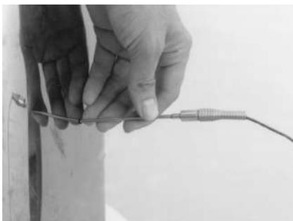
**2** Wearing safety glasses, drill a 1/8" hole all the way through the kiln case and wall.
