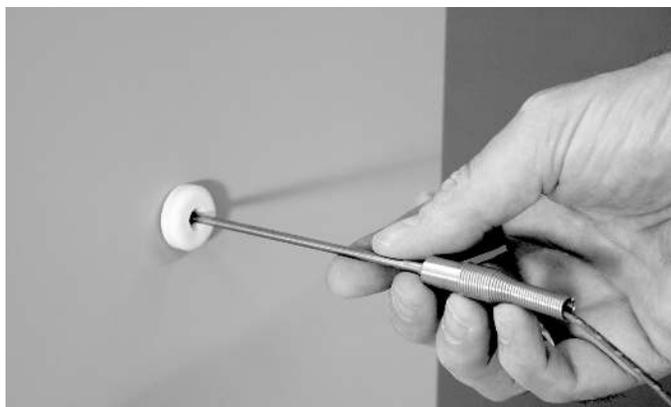
The porcelain insulator that is furnished with the controller is used to mount the thermocouple in a 1/2" hole on the kiln. Do not allow the thermocouple to fall out of the kiln during firing, or the kiln could overfire.
