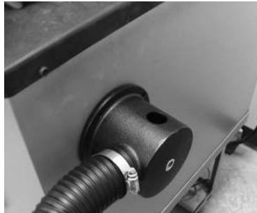
Side kiln mount of collector cup
