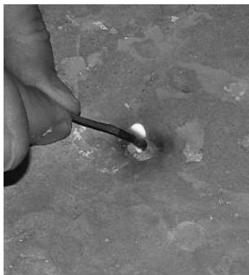
Flame is pulled into the kiln
