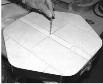
Drill holes in kiln floor with drill bit provided
